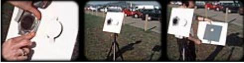
4) Use the duct tape to seal any holes that leak light past the cardboard.
