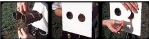
1) First, you should firmly fix the binoculars to a tripod. You can do this with duct tape (what else?).
